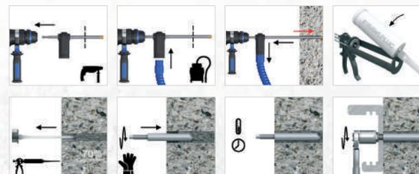
Apply a new and innovative drilling method using our special dustless drill bit. Rawplug's hollow Dustless Drill bit makes every installation easier, cleaner and more durable.
