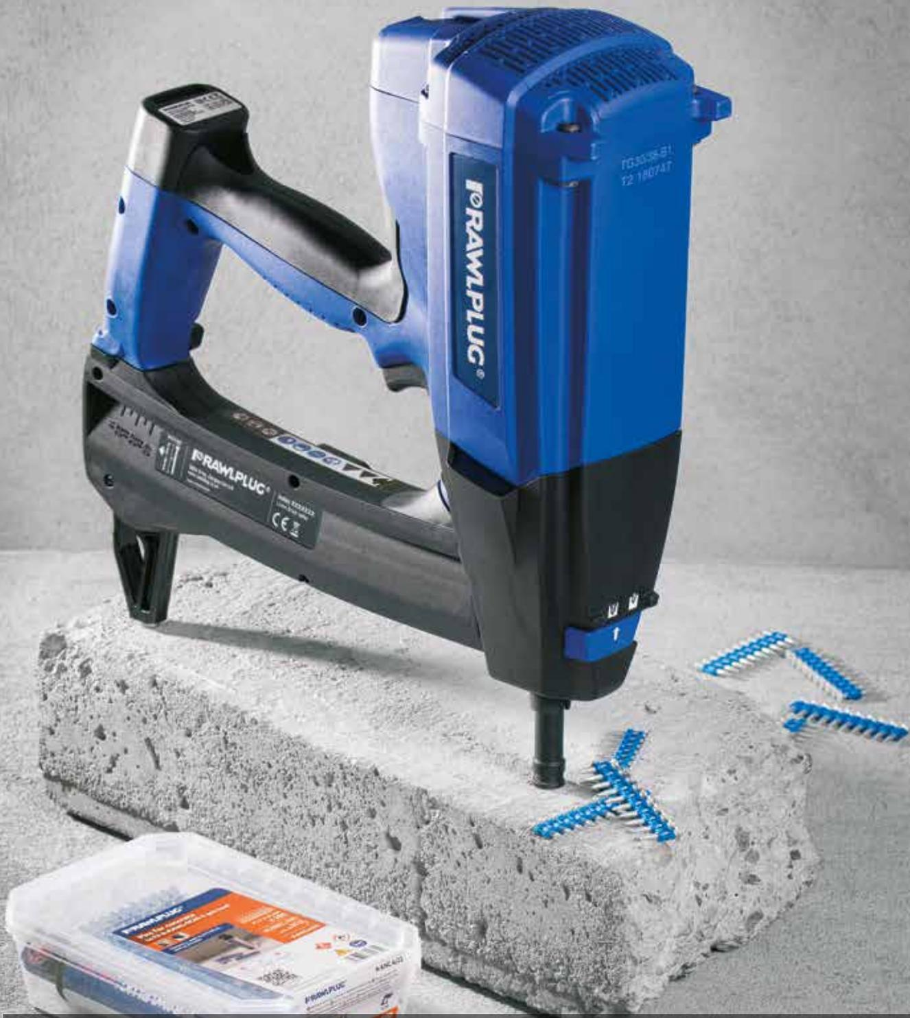
New generation of gas powered nailer for steel and concrete from Rawlplug is capable of securing round head pins in steel and concrete using a combustion Energy of a gas mixture. The fixing is performed in under one second each. If we combine this with battery efficiency of 8000 fixings per charge and charging time of just 30 minutes, the result is a tremendous improvement in jobsite productivity.
