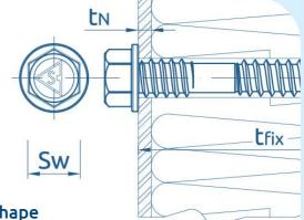
Stainless steel self drilling screw with special drill bit shape designed to provide quick installation in metal constructions made from cold formed sections
